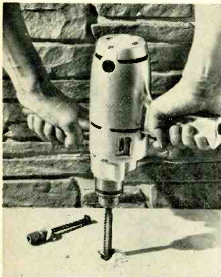
Wen 950 drill with electronic speed control.
