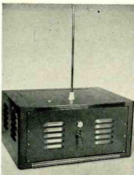
Uhf signals radiated from antenna set up rf field throughout the protected area.
